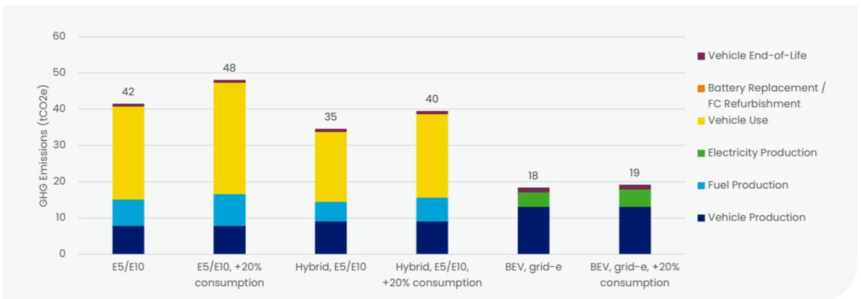
**Figure 27. Impact of fuel consumption on passenger car total life cycle GHG emissions**
