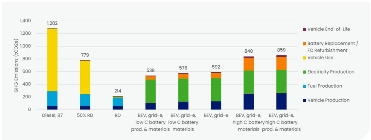
**Figure 22. Impact of battery carbon intensity on artic total life cycle GHG emissions**
