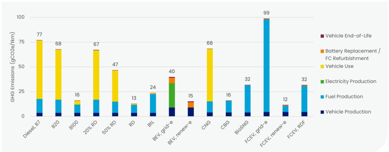
**Figure 13. Total life cycle GHG emissions per tonne-km for articulated truck (30-44 tonne)**
