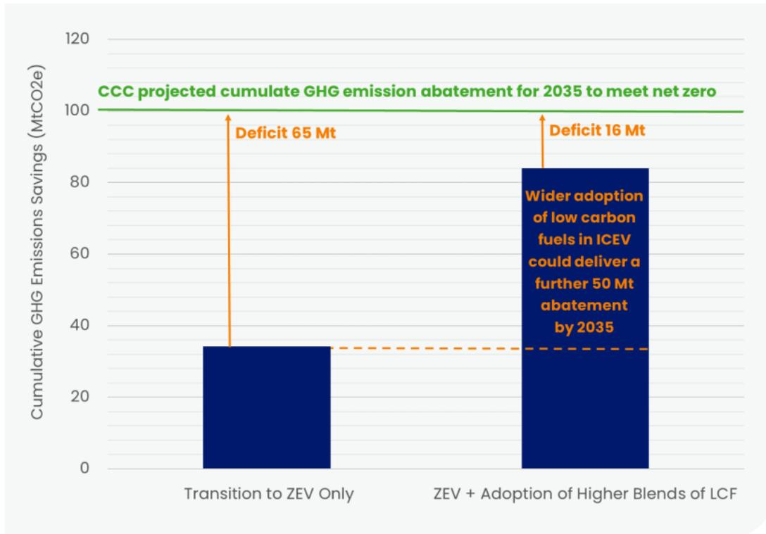
**Figure 1. Modelled GHG emissions savings with and without the adoption of higher blends of low carbon fuels in heavy goods vehicles (HGVs)<sup>1</sup>**
