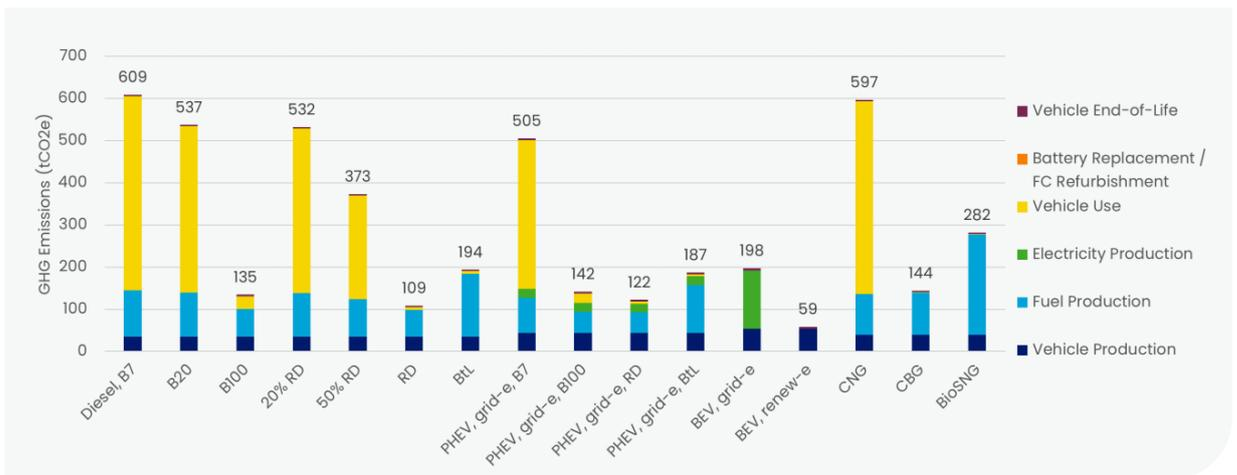
Figure 10. Total life cycle GHG emissions for medium rigid truck (12-32 tonne)
