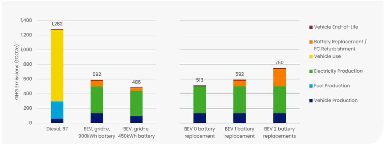
**Figure 21. Impact of battery sizing and replacement on artic total life cycle GHG emissions**
