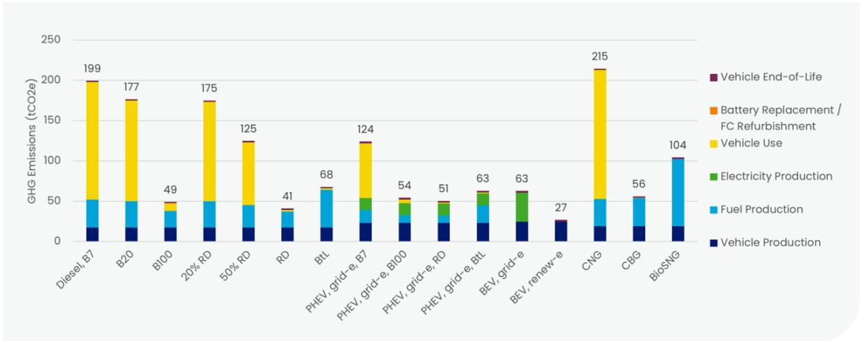
Figure 9. Total life cycle GHG emissions for small rigid truck (7.5 tonne)
