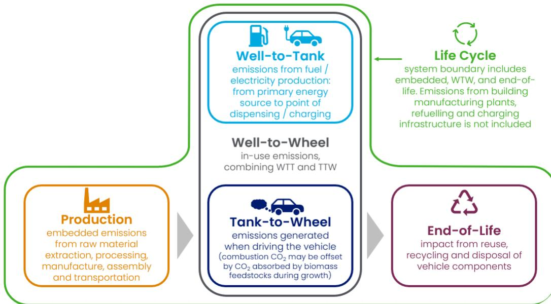
Figure 4. Vehicle life cycle system boundary
