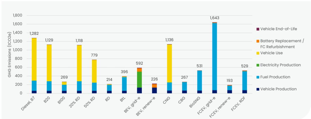
**Figure 11. Total life cycle GHG emissions for articulated truck (30–44 tonne)**
