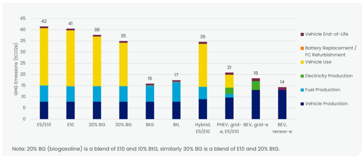
**Figure 7. Total life cycle GHG emissions for medium sized (C-segment) passenger car**
