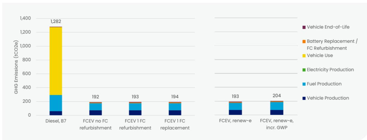
**Figure 23. Impact of fuel cell refurbishment/replacement and hydrogen GWP on artic total life cycle GHG emissions**
